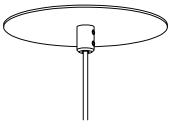
Mounting Option Power 1-2 Octagon Box (By Others) Installed in drywall, wood or concrete ceiling
